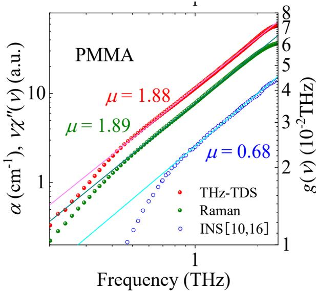
**Fig. 2.** Comparison of the log–log plots of  $\alpha(\nu)$  (red),  $\nu\chi''(\nu)$  (green) and  $g(\nu)$  [10,16] (blue) of PMMA with frequency. The data of  $g(\nu)$  is quoted from previous studies based on inelastic neutron scattering (INS) [10,16].
