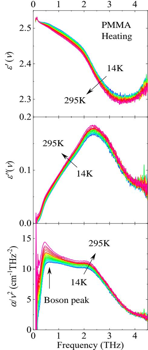
**Fig. 1.** Temperature dependence of the (a) real and (b) imaginary parts of the complex dielectric constants and (c) the BP curve  $\alpha(\nu)/\nu^2$  of PMMA, obtained during the heating process
