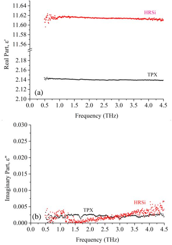
**Fig. 2.** The extracted optical parameters of TPX and HRSi: (a) real part, and (b) imaginary part of complex permittivity.
