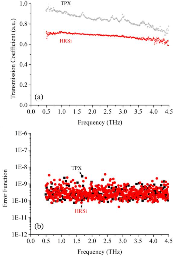
**Fig. 1.** (a) The measured and modelled amplitude of the transmission coefficient of TPX and HRSi, and (b) the error function.
