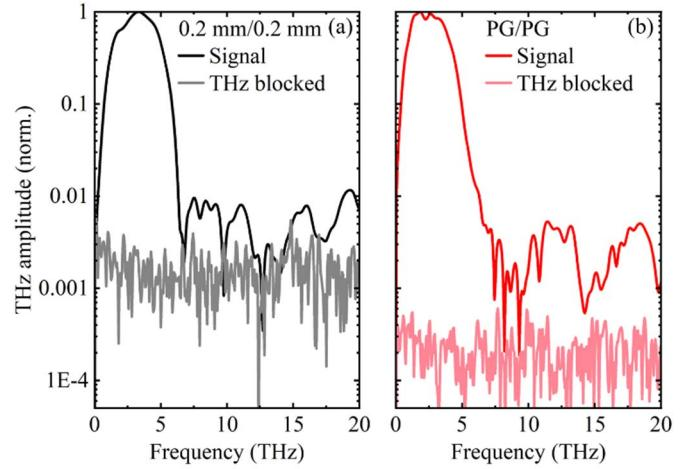
**Fig. 3.** (a) THz spectral amplitude measured with a pair of thin 0.2 mm thick generation and detection GaP crystals. (b) Same measurement performed with a pair of 2-mm thick GaP crystals with a phase (PG) etched on the incident surface to enable non-collinear phase matching conditions. The dashed lines correspond to the noise floor measured by blocking the THz beam.
