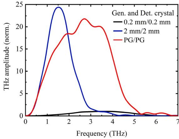
**Fig. 2.** THz spectral amplitude measured with 3 pairs of identical generation and detection GaP crystals having a thickness of 0.2 and 2 mm. A phase grating (PG) on the incident surface of a 2 mm-thick crystal modulates phase matching conditions to enhance THz generation and detection above 2 THz. The THz amplitude is normalized to the total power detected on the balanced photodiodes and then to peak amplitude measured with the pair of thin GaP crystals.
