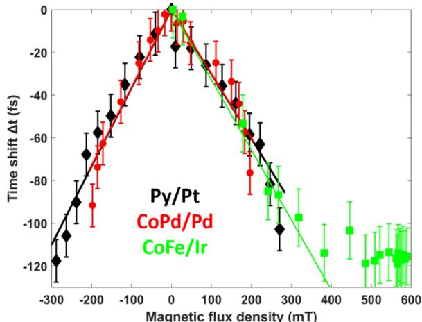
**Fig. 2** Time shift  $\Delta t$  dependence on the magnetic flux density  $B$  for Py/Pt (black dots), CoPd/Pd (red dots) and CoFe/Ir (green dots) nanobilayers. The error bars correspond to the time delay due to a single step of the delay stage. The solid lines are linear fits of the measurement data.
