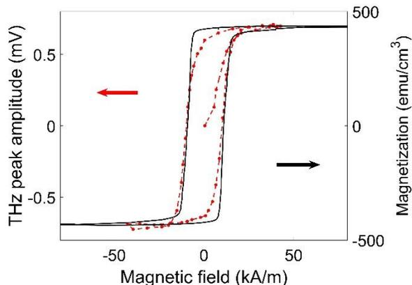
**Fig. 3** Magnetic hysteresis loop  $\mu(H)$  (black solid lines) of a FeCo/Ir bilayer and magnetic field dependence of the THz peak amplitude starting from the demagnetized state (red symbols). By recording the THz transient from a demagnetized FeCo/Ir bilayer, the initial virgin magnetization hysteresis curve can be extracted.
