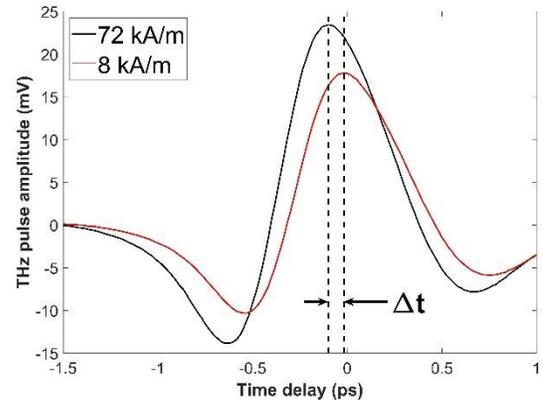
**Fig. 1** THz transients generated by laser illumination of a Ni<sub>80</sub>Fe<sub>20</sub>/Pt bilayer using a train of 100 fs laser pulses, recorded at two external magnetic field intensities. The THz transient recorded at a higher magnetic field (black trace) shows a clear time shift by  $\Delta t \sim 110$  fs with respect to the transient recorded at low field (red trace). Both transients were measured at a fixed detector position and the same intensity of optical excitation.
