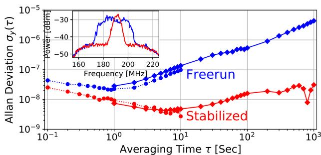
Fig. 4. Allan standard deviation of CO-stabilized THz-QCL. Inset: RF spectra of heterodyne beat signal of frequency-locked (red) and free running (blue).
