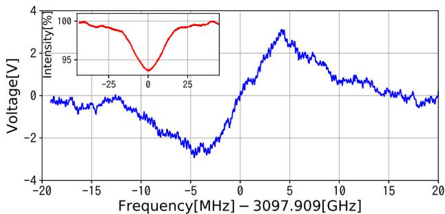
Fig. 3. First-derivative signal of rotational-transition spectrum of CO molecule. Inset: Linear absorption spectrum of  $J = 27 \leftarrow 26$  transition.
