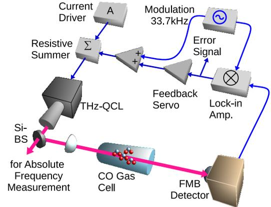
Fig. 2. Experimental setup for THz-QCL frequency stabilization.
