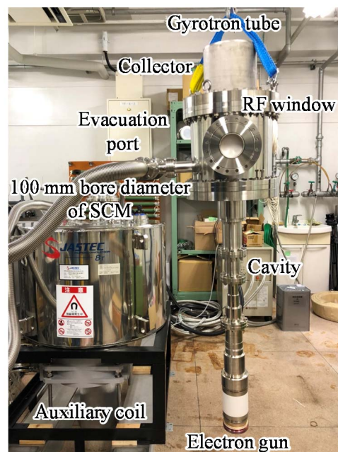
Fig. 2. A photograph of a 100 mm bore diameter of SCM and assembled gyrotron tube.
