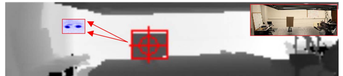
Fig. 1. LiDAR contour scan of the optical table and room. The red crosshair signifies the pattern recognition algorithm located the target to record a sub-THz reflected intensity image shown in the inset (left) that identifies two targets. The grey scale of the LiDAR image is proportional to distance and the dark blue indicated two strongly reflecting targets. Right inset is an optical comparison from the vantage point of the LiDAR.
