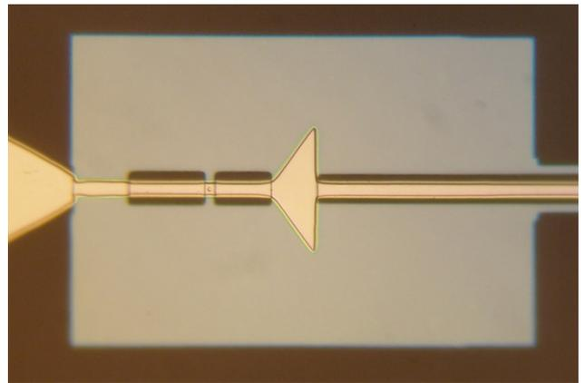
**Fig. 1.** Photo of the SIS mixer element inserted in the planar structure formed by segments of coplanar and microstrip Nb/SiO<sub>2</sub>/Nb lines.
